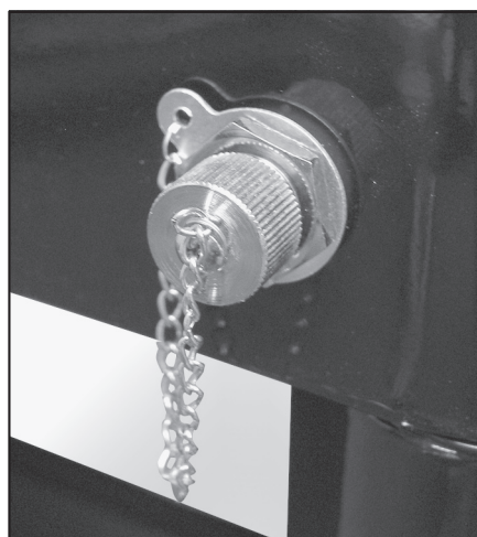
Step 8: Place drain plug through hole. Threads facing back of cooler. Slide rubber washer and nut over threads. Tighten securely.
